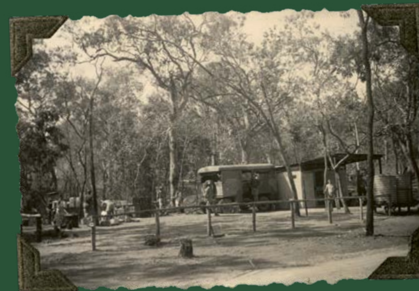
Wiles Travelling Army Field Kitchen at Rollingstone Army Camp, Queensland 1943. The mobile kitchen cooked meals for 100 to 500 men, and featured steamers, ovens and a 40-gallon hot water tank.
